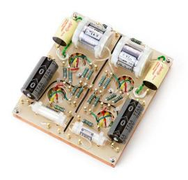
Modular design is one of the iconic designs of Audio Note new generation amplifiers. It is now fully symmetric and independent for left and right channels at G-1000. With the help of well distributed capacitor groups, the signal loops are shortened at the line amplifier unit. For best matching with solid state or low input impedance power amplifier, G-1000 output impedance is  $600\Omega$  and cutoff frequency reaches 18.5Hz (under  $20k\Omega$  load).
